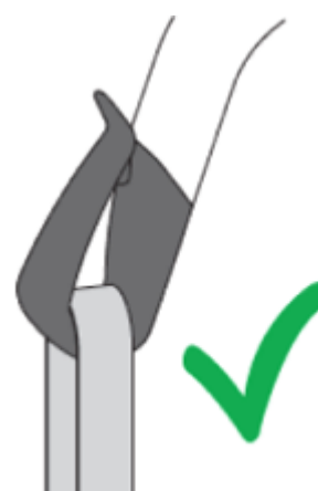
PICTURE 2 - CORRECT SLING LOOP ATTACHMENT
