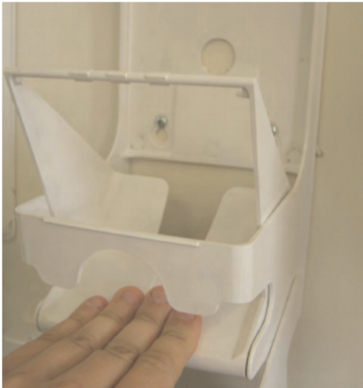
As from stage 2, Use the bottom of the dispenser to lever the inside mechanism that releases the second roll
